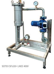
The SFU+ is equipped with 2 pressure gauges. As soon as there is sufficient pressure difference, the filter bag is contaminated and must be replaced. The whole is beautifully assembled in a stainless steel frame. In short, a 'plug-and-play' unit.
